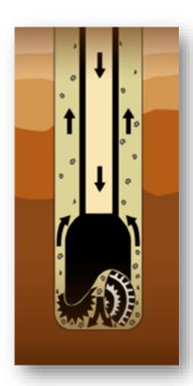
The crew sets up the rig and starts the drilling operations. First, from the starter hole, the team drills a surface hole down to a pre-set depth, which is somewhere above where they think the oil trap is located. There are five basic steps to drilling the surface hole:
